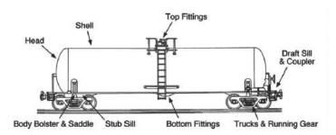
The tank is made of steel plate, 7/16 of an inch thick. An oil tank car is typically loaded from the top valve and unloaded from the bottom valve. Loading or unloading each car may take several hours, but multiple cars in a train can be loaded or unloaded simultaneously.
